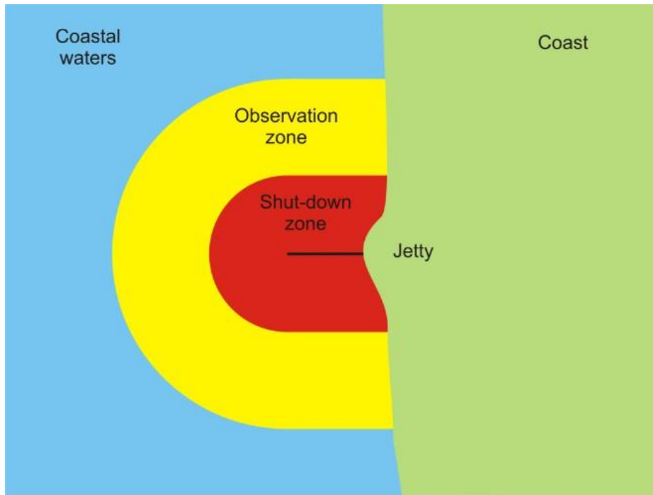
Figure 1 – Diagram showing example “observation” and “shut-down” zones around a jetty [Ref.4, Ref 15].
