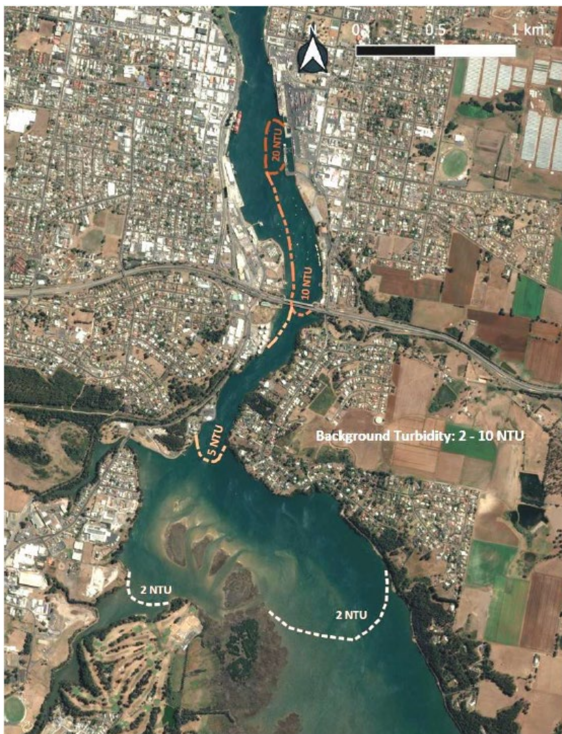
Figure 9: Predicted plum extent and turbidity above background levels on a peak flood tide (figure 6-7 in the EIS)
