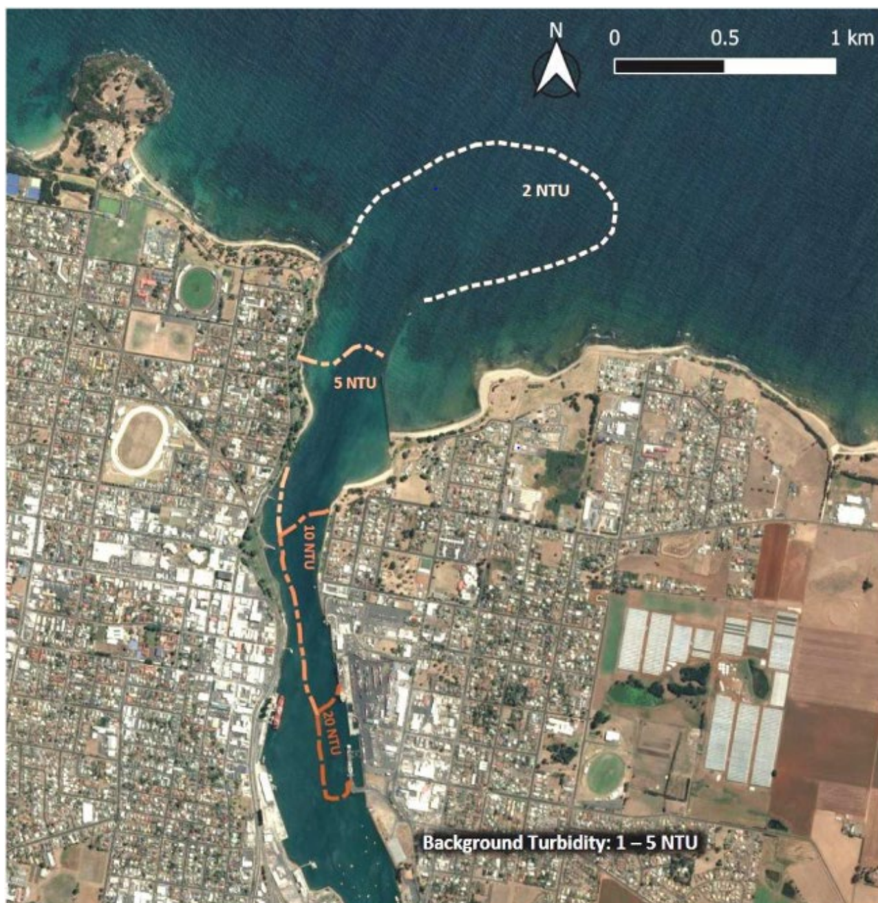
Figure 8: Predicted plume extent and turbidity above background levels on a spring ebb tide (figure 6-6 in the EIS)
